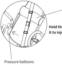
Hold the pressure balloon with your hand and squeeze it to inject air into the 18 # waist pad.
