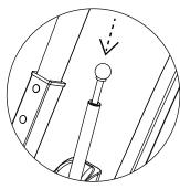
Press down the ball bar, adjust it forward and backward to a comfortable angle, and insert the 21 # pull ring bolt.
