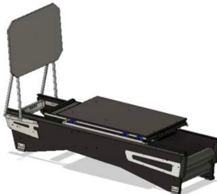
Kickplate Structure (Foot-End)
