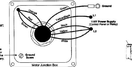
Magnetek TENV Motor: Clockwise Rotation (for counterclockwise rotation, interchange black and red leads)
