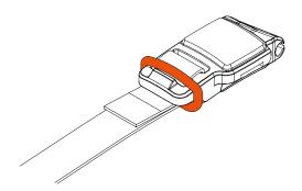
Note This illustration is only valid for the SNAP buckle piping (article no. F6030) and visualises how the webbing is fixed to the buckle with a rubber ring.
