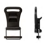
Opening mechanism Webbing width 25 mm Weight ca. 14 g Dimensions (L×W×H) 44,5 × 33,9 × 12,4 mm Material PA66GF15 Static breaking load 40 kg Colour black Assembly
