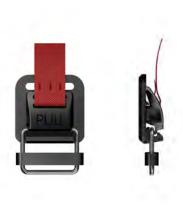
Opening mechanism pull Webbing width  $25\,mm$ Weight ca. 13 g Dimensions (L×W×H)  $49,2 \times 34 \times 11,8$  mm (incl. D-ring) Material PA6, PA66GF15, stainless steel Static breaking load 30 kg Colour black
