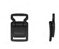
lift Webbing width 20 mm Weight ca. 7 g Dimensions (L×W×H) 43,1 × 26,8 × 8,9 mm Material PA66GF15 Static breaking load 15 kg Colour black Assembly
