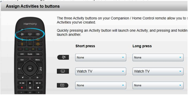
With a single press of the Watch TV button the receiver, TV, and ZapperBox are turned on. The receiver and TV are set to the proper inputs and an over-the-air TV station will be displayed via the ZapperBox. A single press of the Off button will turn off all 3 Devices.
