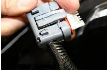
Important Note – Cut off or Cover the terminals that are not used with heat shrink, they can cause short circuit!
