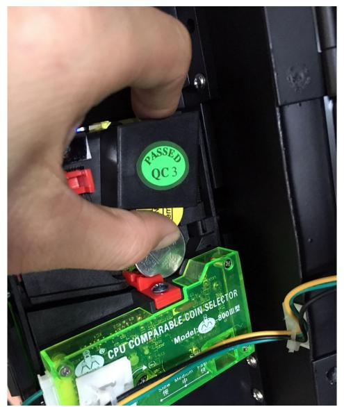
1) If put \$1 coin in this place, then the coin acceptor can accept \$1 coin.
