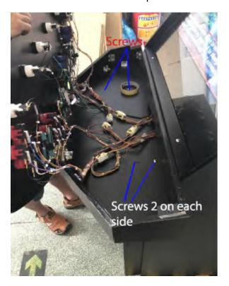
(2) Connect the joystick and button wires to main body, please see below:
