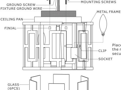
Place the glass inside the metal frame and secure it with the clips.
