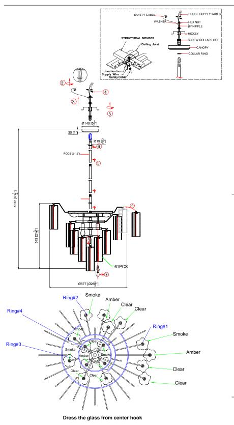
1.For ring#1,the pattern of glass arrangement is 2pcs of clear glass+1pc smoke glass +1pc amber glass.
