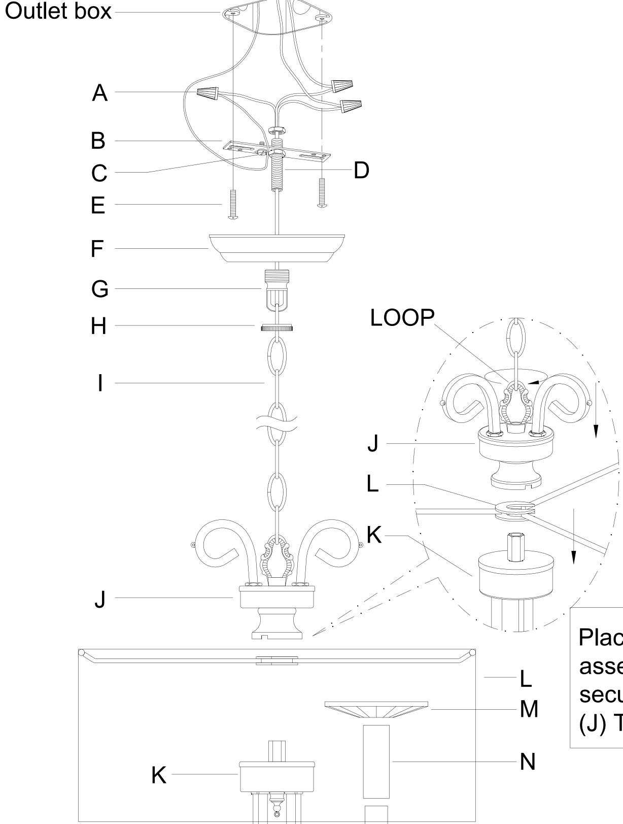
Place the (L) Fabric shade and (J) Top assembly on top of (K) Frame then secure by tightening the loop on the (J) Top Assembly.
