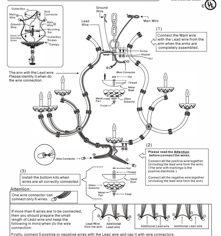
Secondly, do the same for the rest of wire connection. Please make sure all the small length Lead wire
