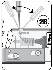
To pump master cylinder, insert a flat tip screwdriver into the round hole near the front of the actuator cover (See 1A). The screwdriver should be at the lowest angle possible to the actuator so that it slides in front of the e-stop bracket (See 1B). Screwdriver tip MUST BE IN FRONT of the e-stop bracket and NOT in the slot on the e-stop bracket (See 2A). Push the screwdriver forward and back to pump the master cylinder. (See 2B).
