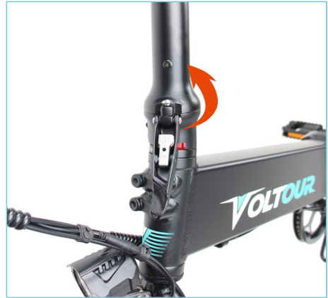
Step 6: Fold the latch up to lock the stem.
