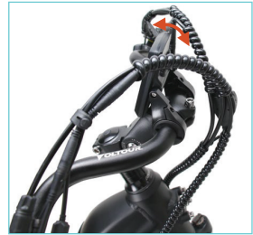
Step 6: Adjust display to proper position.
