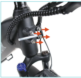
Step 1: Remove the four screws.
