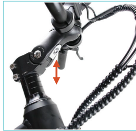
Step 5: Adjust handlebar height to proper position.
