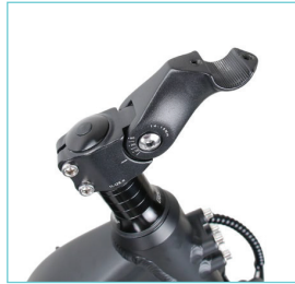
Step 2: Screws and rubber gasket removed.
