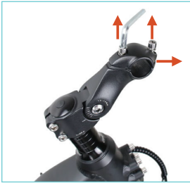
Step 1: Remove handlebar screws and rubber gasket.
