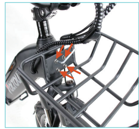
Step 3: Tighten the four screws.
