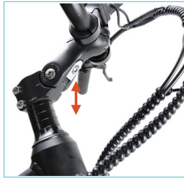
Step 5: Adjust handlebar height to proper position.
