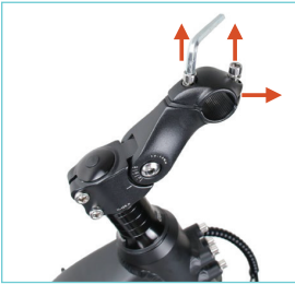
Step 1: Remove handlebar screws and rubber gasket.
