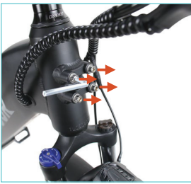
Step 1: Remove the four screws.
