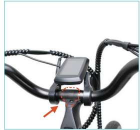
Step 3: Put handlebars and rubber gasket in proper position.
