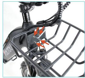
Step 3: Tighten the four screws.
