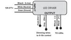
After installing the luminaire, make wiring connections as shown in the wiring diagram.
