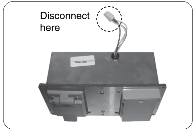
Fig. 40-2 Slightly pull out box and disconnect wire harness
