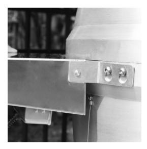
2. Once the shelf brackets are properly positioned over the fasteners, tighten the fasteners with the included #5 mm allen wrench.
