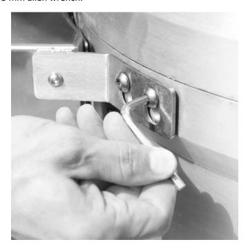
3. Underneath the shelf, you will find a shelf leveling / stabilizing screw. This screw holds tension against the grill body leveling the shelf and holding it securely in this position. Tighten this screw either by hand or using the #6 mm allen wrench. When complete, the shelf should be level. See below:
