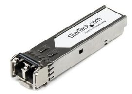
The SX-ST is a Palo Alto PAN-SFP-SX compatible fiber transceiver module that has been designed, programmed and tested to work with Palo Alto brand switches and routers. It delivers dependable 1 GbE connectivity over fiber cable, for 1000BASE-SX compliant networks, with a maximum distance of up to 550 m (1804 ft).
