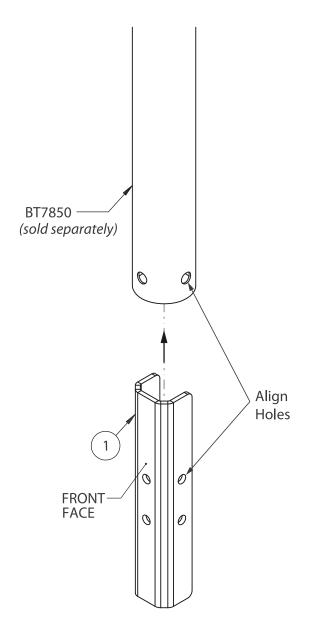
**NOTE:** Keep the middle face of the internal pole joiner facing the front side where the screen/s are to be mounted.
