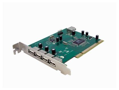
This PCI-based High Speed USB 2.0 Adapter Card adds seven USB 2.0 ports (1 internal USB A Female, 2 internal USB motherboard header, and 4 external USB A Female) to your PCI-capable PC.
