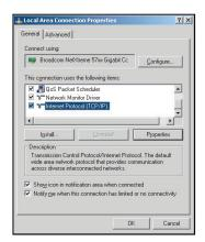
6. Type in the IP address and Subnet mask, then press "OK".
