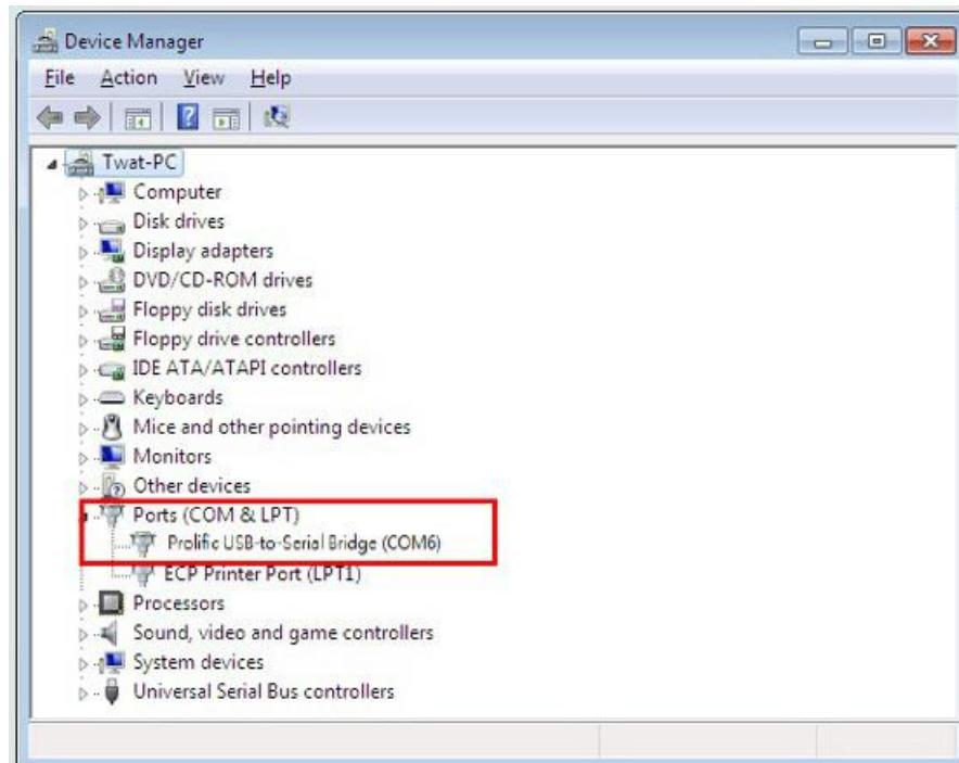
2. Choose **Serial** and the corresponding COM port as the communication port. In this given example, COM6 is selected.
