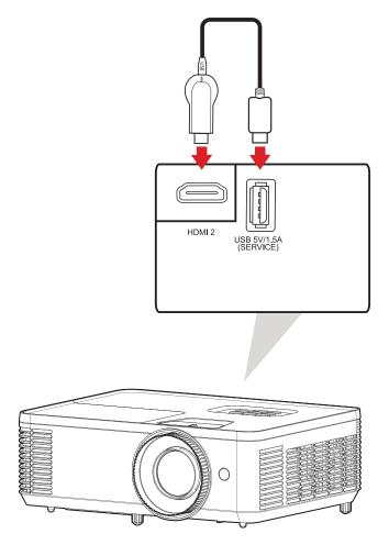
**NOTE:** USB Type A supports 5V/1.5A power output for HDMI dongle charging.
