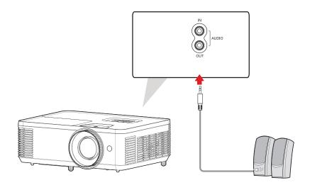
Additionally, you can connect to the **AUDIO IN** port with your device to use the projector's audio output.
