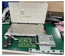
LCD module(together with their casing) is only left after all other parts like electronic units and casing have been removed.
