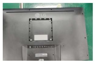
Re-overturn the set and disaaemble screw 4EA and disassemble the PCB
