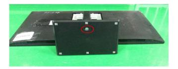
Push button and lift the stand body and remove the screw(4EA)
