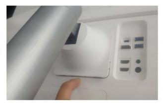
Remove 4 x screws to disassemble the back cover. (Tool set up : Screw driver with "+" tip.)
