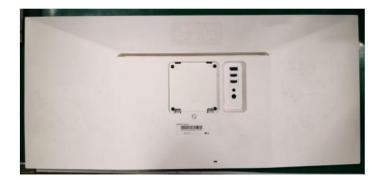
Re-overturn the set and disaaemble screw 4EA and disassemble the PCB
