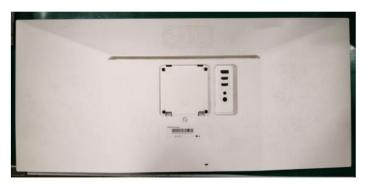
Re-overturn the set and disaaemble screw 4EA and disassemble the PCB
