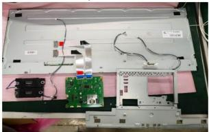
LCD module(together with their casing) is only left after all other parts like electronic units and casing have been removed.
