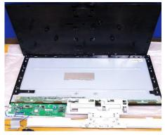
LCD module(together with their casing) is only left after all other parts like electronic units and casing have been removed.
