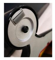
Push button and lift the stand body and remove the screw(1EA)
