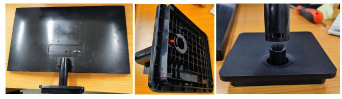
remove the screw and lift the stand body
