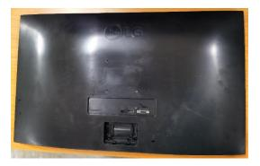
Re-overturn the set and disaaemble screw 2EA and disassemble the PCB
