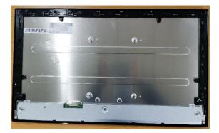
Re-overturn the set and disaaemble screw 4EA and disassemble the PCB
