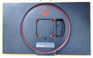
Overturn the set and disassemble the latches of three edges
