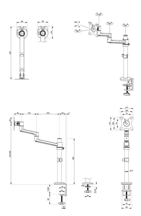
Neomounts Measuring unit: mm
