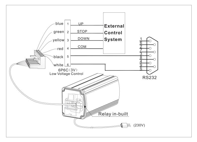
Note: Please do not connect the RS232 line all the time to prevent from damage to the relay
