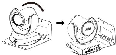
3. Pass cables through A or B hole first. Connect cables with camera.
