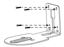
3. Then, assemble the L-mount brackets  $\boxed{\mathsf{A}}$  +  $\boxed{\mathsf{B}}$  with screws (included in package).
