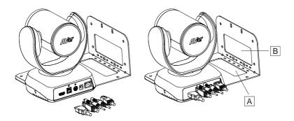
4. Turn the camera to face the front side. Install the second screw and tighten both screws.
