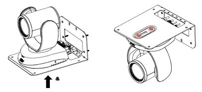
5. Find suitable screws to fix the camera mount to the ceiling.
