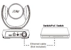
Or connect a CAT 5e FTP cable (not included) to the PoE Switch or Ethernet.
