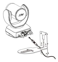
6. Use the remaining screws (included in package) to secure the camera on the L-mount bracket.
