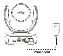
Connect the included power adapter and power cord to a wall outlet.
