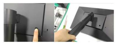
Remove 4 x screws to disassemble the back cover. (Tool set up : Screw driver with "+" tip.)
