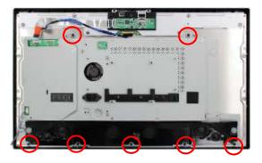
Remove 11 x Screws for the main PCB and Power PCB
