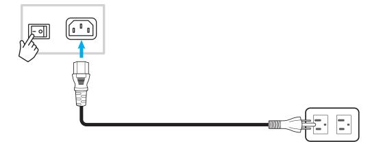
Press the **Power** button to turn the panel on. The LED indicator light turns blue, indicating it is ready to use.
