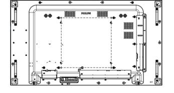
M6 \* (10+X) mm (X=Thickness of Wall mount BKT) 55BDL4107X/55BDL4105X: 400mm x 400mm
