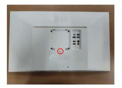
Overturn the set use jig to disassemble backcover
