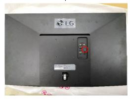
Overturn the set and disassemble the latches of top edges and use jig to disassemble backcover
