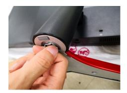
Disassemble the top cover and stand body and remove the screw(1EA)
