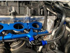
28. Install the two provided standoffs using the provided screws to secure them to the metal brackets in the car.
