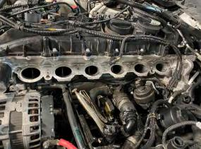
23. Depending on the date of production trimming of manifold may be required, manifolds that come with the 5 tabs circled in red below will require trimming/grinding.
