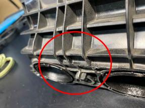
25. With the o-rings still removed from the manifold push the bolts out of the manifold and place port injection plate against the face of manifold. Then while holding firmly inspect for clearance. Minor grinding might be needed to remove corners off some ribs on the manifold so that plate can meet flush against manifold.
