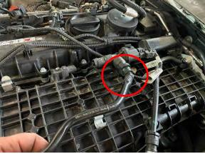
15. Disconnect all wires from the sensors shown below circled in red.
