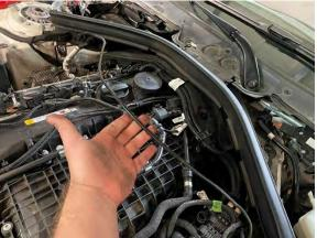
8. Remove the rubber trim located at the back of engine bay by pulling forward on rubber starting at one side.
