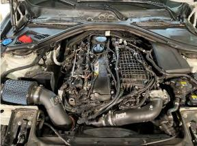
4. Remove the plastic cowl cover on both drivers and passengers side using a 10mm socket to unlock the locking tabs.
