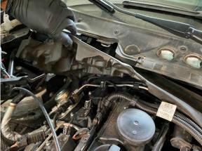
13. Remove the electrical connectors from the DME working from front of car to back of car, each connector has a release that gets pushed down then lever pulls forward releasing the connector from the DME. Also remove cable holding clip by pressing both releases and pushing up.
