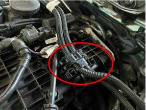
14. Remove the emissions vacuum hose by removing 1 T20 screw and releasing the quick connect at the other end of the hose.
