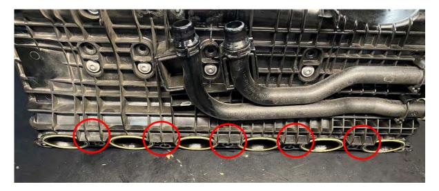
24. For manifolds that require grinding, start by removing all 6 o-rings to prevent damaged. With o-rings removed cut each of the tabs flush with the manifold (note the alignment tabs do not need to be removed).
