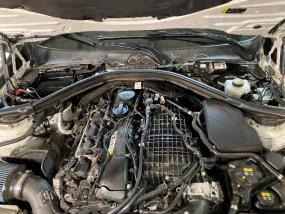
5. Remove the rubber trim on top of the struts located on both the drivers and passengers' sides by removing the push pins.
