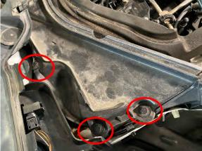
12. Remove the cowl tray and sound dampening foam from the engine bay.
