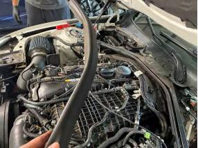
9. Remove the two covers located in the center of the cowl allowing access to the e-torx below.
