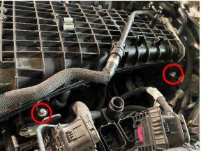
22. Lift the manifold towards the driver side of the car away from the cylinder head and disconnect the two coolant lines for the intercooler by pulling the release clips away from the hose until they lock then pulling firmly on hose. Once disconnected remove the intake manifold from the car.
