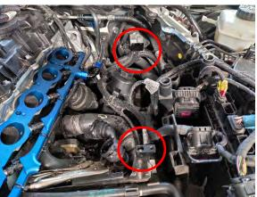
29. Reinstall the factory o-rings in the manifold and install the manifold in the reverse order of removal.
