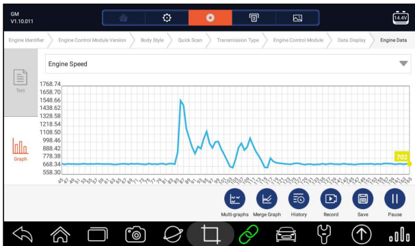
Figure 5-21 Sample PID Graph Screen
