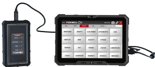
Figure 4-3 Sample USB Connection
