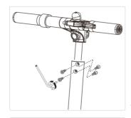
Put the handle bar set into the folding head tube, and keep the brake in the front.
