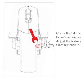
Clamp the 14mm nut from the brake, then loose 9mm nut aside.
