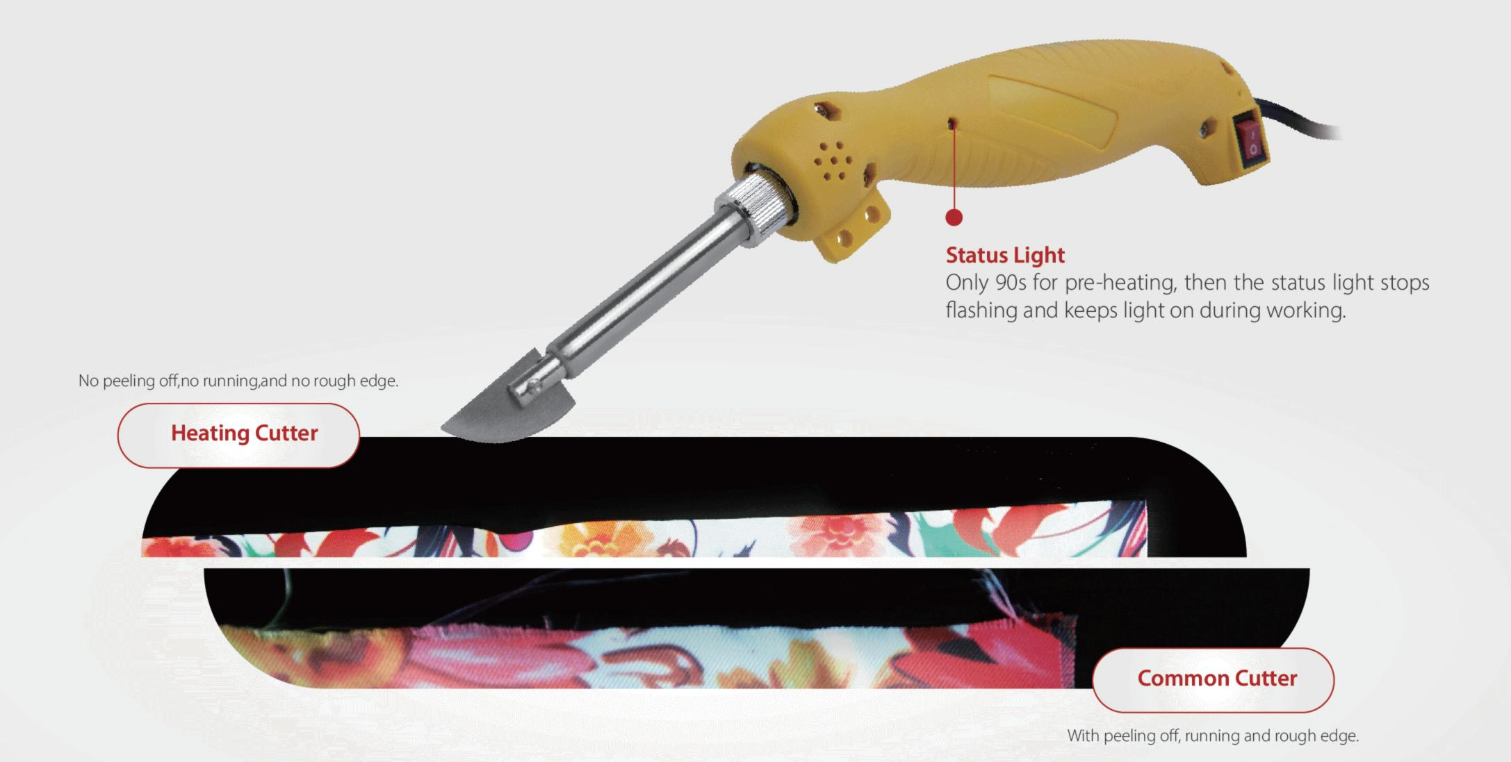
Heating cutter, specially designed for chemical fabrics, synchronized cutting and ironing, no peeling off, no running, no rough edge, to facilitate the post-processing, easy to operate.
