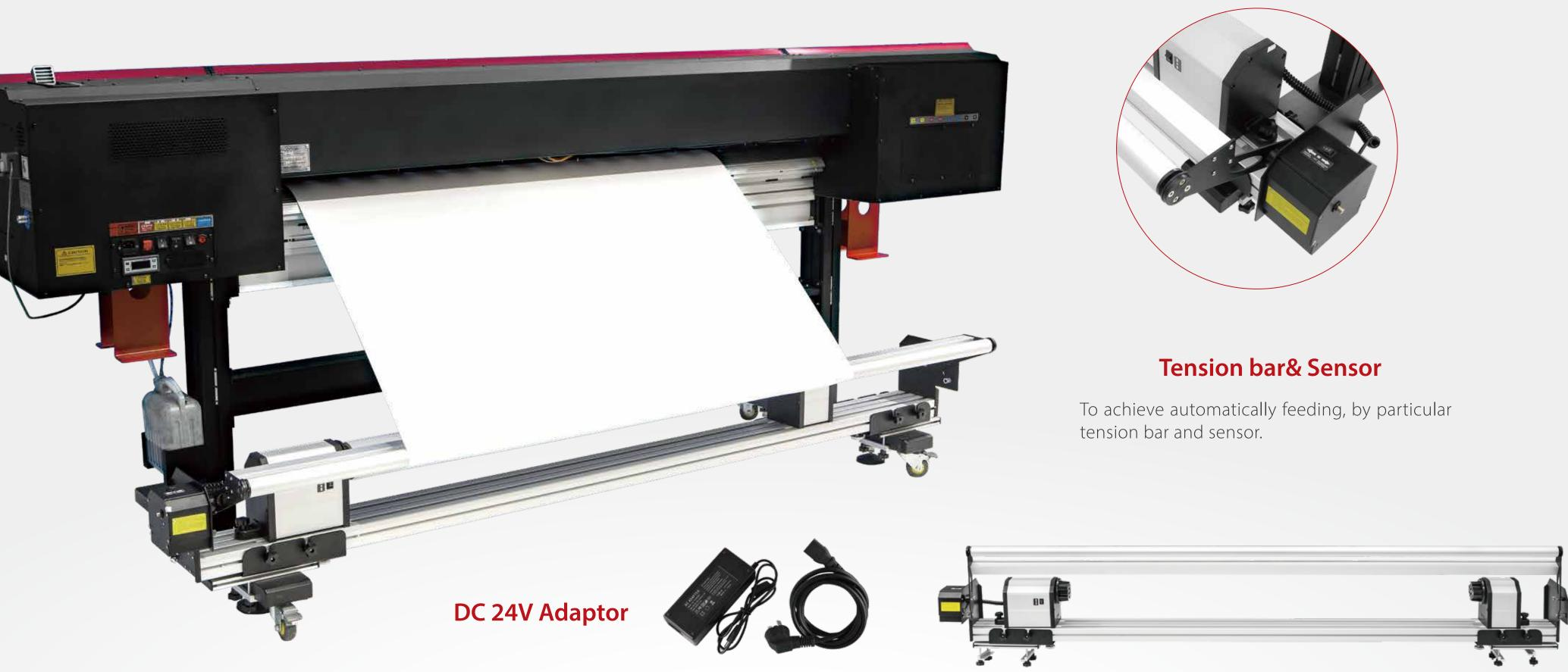
Feeding system with inductive tension and track design in domestic. Motor drive, neat feeding, durable life. Adopt the inductive tension structure, ensure stretch the graphics smoothly in the feeding process, also applies to heavy media.
