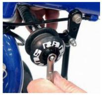
Rotate the idler assembly forward until chain is taught. If the bottom chain contacts the top chain, remove a link using a chain link. Do this at the cheater link shown in the picture below.
