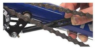
In most cases it will be necessary to replace or modify your support arm give the proper range of adjustment for the idler bracket. If your arm is of the tubular steel type it can be adapted by adding 5mm holes to it. If your arm is of the aluminum type it will have to be replaced with the tubular steel type and adapted.
