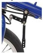
Reinstall the idler on the axle positioning the chain over the idler as shown in the picture. Reinstall the washers and cap nuts.
