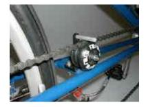
Idler mount is machined to saddle frame tube.
