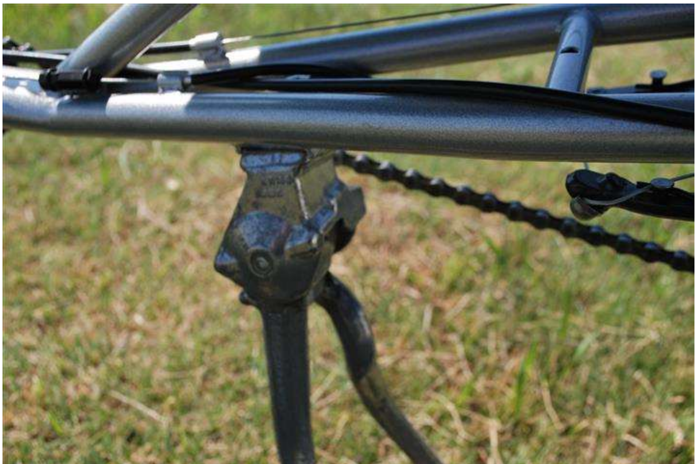
Stock equipment for 2014: a double leg Kick Stand, mounts to integrated pad on frame.
